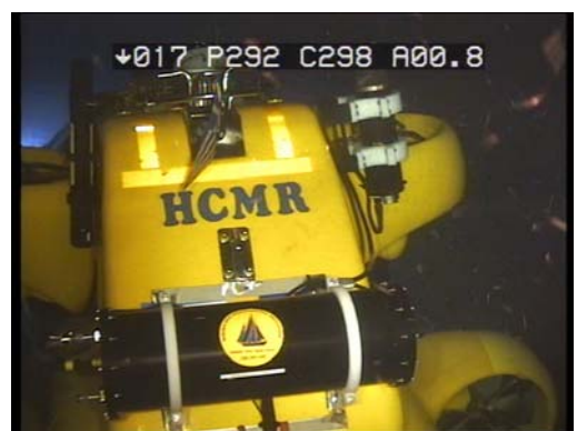
Figure 3: photo of TETHYS-Gemini prototype during deployment onboard the HCMR Thetis submersible at a depth of approximately 300 meters in the Santorini Caldera.
